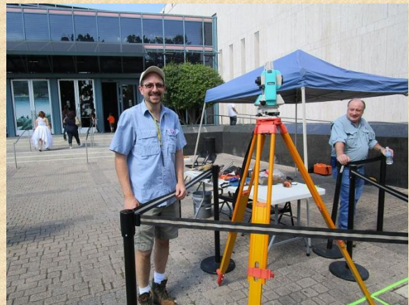
Tony Scott from HRA Gray and Pape demonstrated the use of a total station on archeological sites.
